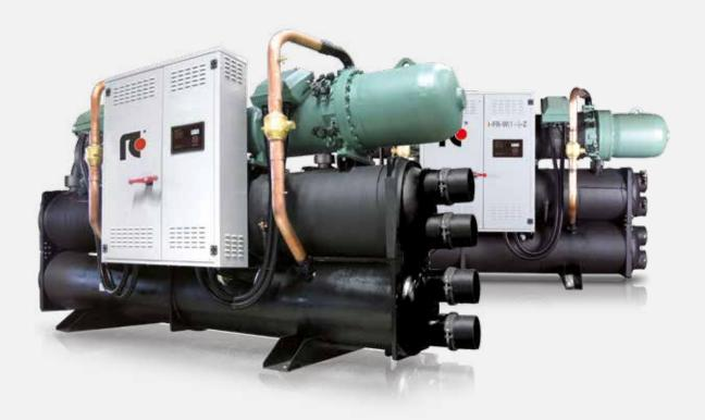
i-FR-W is the RC brand water cooled chiller with 1+i innovative logics that combines fifixed speed and variable speed screw compressors, thus ensuring continuous modulation of loads and a perfect leaving water stability.
